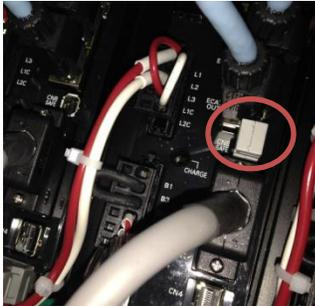
2. Removing jumpers by hand can cause the latch to break. Recommended practice is to use a screw driver. The latch is on the left side.
