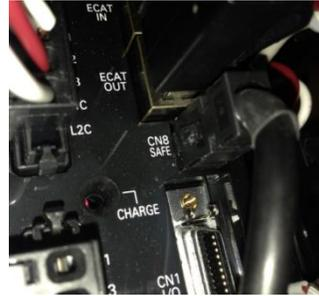
4. Up to 4 G5 servos drives can be daisy chained. Add EtherCAT cable to connect.
